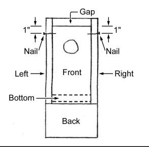
Step 10 Drill a 3/16" hole through the right panel into the front panel. Start the hole about 2" from the bottom of the right panel, and angle the hole slightly downward.
